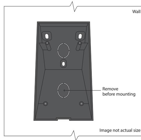
4. On the mounting bracket, you will need to remove the oval-shaped cable hole to ensure that the time clock cords can be pulled through.
